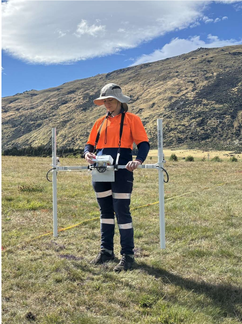
Southern Geophysical conducting a magnetic gradiometer survey
